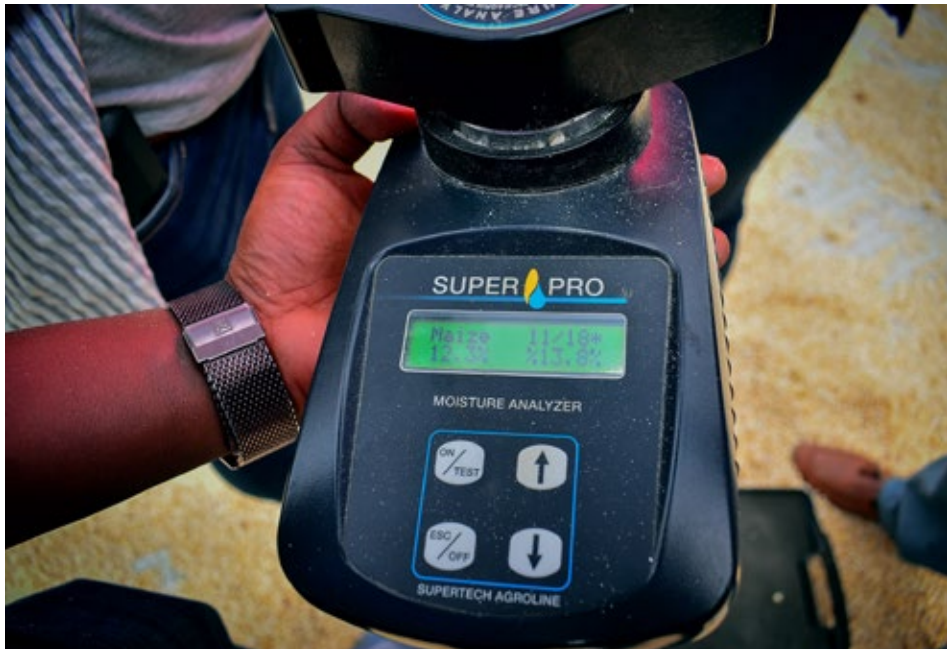
Figure 6. Tom Bowen demonstrating how a maize moisture analyzer works: Photo by AZE world
